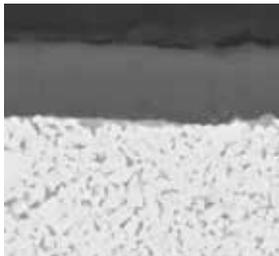
PVD coated S05–S15 carbide substrate for finishing to medium application of super alloy material but also stainless steel. Good wear resistance in a wide application field.
