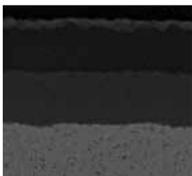
CVD coated K10–K25 carbide substrate. Optimized for medium to roughing operation of cast iron. Improved wear resistance and toughness at high cutting speed.
