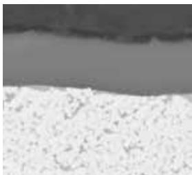
PVD coated M20–M30 / S05–S20 carbide grade for finishing to medium machining of stainless steel and high-alloyed materials. High-performance grade with high wear resistance and residual stress offer a wide range of applications.
