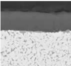
PVD coated S05–S15 carbide substrate for finishing to medium application of super alloy material, stainless steel and aluminum. Good wear resistance in a wide application field.
