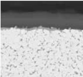
PVD coated N05–N20 carbide substrate for finishing to medium application in aluminum material. Coating only on the top face, in combination with the aluminum chip breaker, prevent build up edge and gives a smooth cut.
