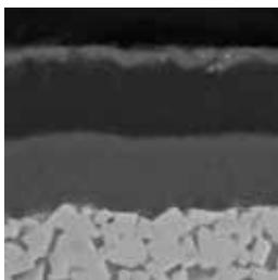
CVD coated P20–P40 carbide grade for roughing operation of steel and casting steel. Optimal performance of wear resistance and toughness for a wide application field.
