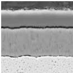
CVD coated P20–P30 carbide grade for medium operation to roughing of steel and casting steel. Optimal performance of wear resistance and toughness for a wide application field.
