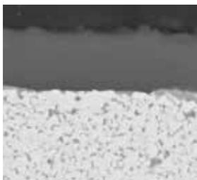
PVD multilayer coated M20–M40 / S15–S25 / P10–P30 carbide substrate for finishing to medium application of stainless steel, super alloy and steel (milling). Good wear resistance and thermal stability in a wide application field.
