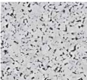
Uncoated N05–N20 / K05–K20 carbide substrate for fine to medium application in aluminum and other materials.
