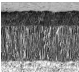
CVD coated K10–K25 carbide substrate. Optimized for medium to roughing operation of cast iron. Good wear resistance and toughness at higher cutting speed.
