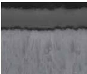
CVD coated M10–M20 carbide grade for finishing to medium application in stainless steel. High wear resistance and capability against plastic deformation at higher cutting speed.
