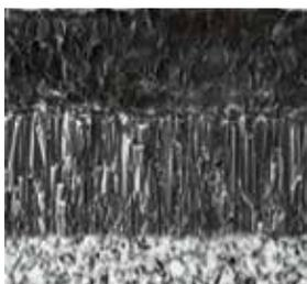
Thick Al<sub>2</sub>O<sub>3</sub> CVD coated K10–K25 carbide substrate. Optimized for medium to roughing operation of cast iron. Higher wear resistance and toughness at higher cutting speed in combination with TC chip breaker.
