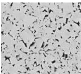
Uncoated N10–N30 / K10–K30 carbide substrate for medium application in aluminum and other material.
