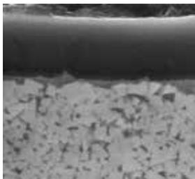
PVD multilayer coated M10–M25 / P10–P30 carbide substrate for finishing to medium application of stainless steel, super alloy and steel (grooving/milling). Optimized coating stability for higher wear resistance and thermal stability in a wide application field.
