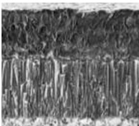
CVD coated K05–K20 carbide substrate. Optimized for medium operation of cast iron, special nodular cast iron and hard steel at high cutting speed.
