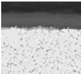
PVD multilayer coated S05–S20 carbide substrate for finishing to medium application of super alloy material but also stainless steel. Good wear resistance and thermal stability in a wide application field.
