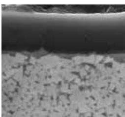
PVD multilayer coated M10–M25 / P10–P30 carbide substrate for finishing to medium application of stainless steel, super alloys and steel (grooving/milling). Optimized coating stability for higher wear resistance and thermal stability in a wide application field.
