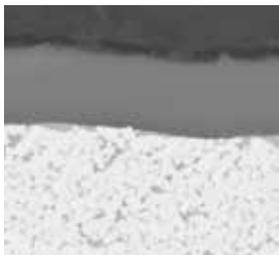
PVD coated M10–M25 / P10–P30 carbide substrate for finishing to medium application of stainless steel and steel (milling). Good wear resistance in a wide application field.
