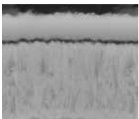
CVD coated M15–M35 carbide grade for medium to roughing operation in stainless steel with wide application field. High wear resistance and capability against plastic deformation at higher cutting speed.
