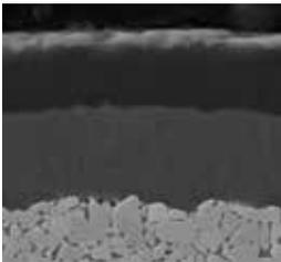
CVD coated P10–P20 carbide grade for finishing to medium operation of steel, casting steel and high chrome material. Outstanding performance under high cutting speed and temperature with excellent wear resistance.
