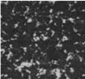
Uncoated N01–N10 brazed PCD grade for fine-finishing operation of aluminum alloy less than 12% Si, composites, copper/magnesium and other alloys. Medium grain size grade with good wear resistance for a wide application field.
