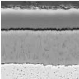
CVD coated P10–P20 carbide grade for finishing to medium operation of steel and casting steel. Outstanding performance under higher cutting speed and temperature with excellent wear resistance.
