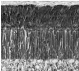
CVD coated K05–K15 carbide grade for finishing cast iron material, special grey cast iron. Excellent wear resistance in higher cutting speed and dry machining.
